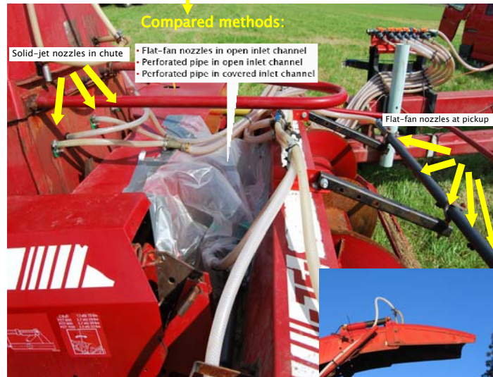
New method, which improved the evenness of application. When the flat fans above were replaced by solid jets, the losses were also reduced.
