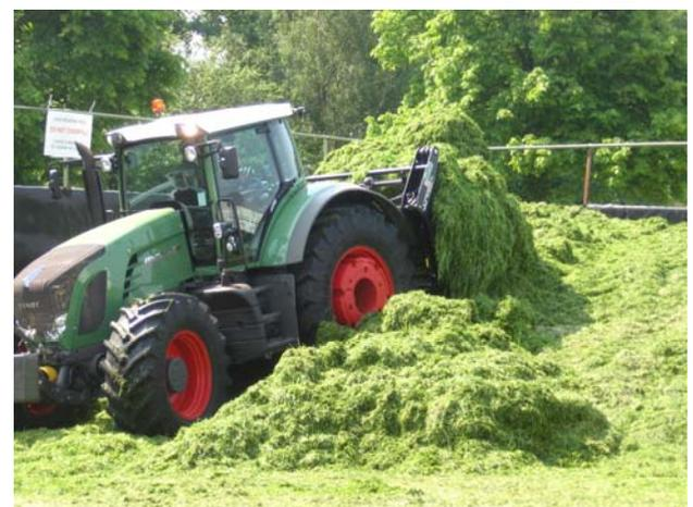
One example of working chain involved in model is loader wagon. Loader wagon method's capacity is 2-2,5 ha in an hour, when transport distance between field and storage is one kilometre. One person drives tractor loader wagon combination and second person levels load and compact it in bunker silo using tractor with loader. Usually before harvesting phase two or three mowing working width are combined into one swath with windrower.
